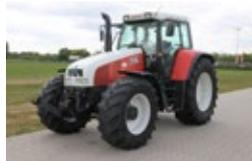
**Steyr S120 SUPER SIX** Bj. 2002, 85 kW, 116 PS, 11.795 Std., 6 Zylinder, 24+24, 40 km/h, 540/540E/1.000/1.000E U/min, Klima, 2 x DW, Druckluft, FKH, EHR, **21.500 €**
